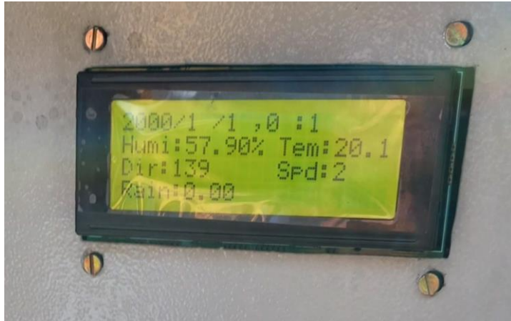
Figure 2: Screen shot of the data seen on the Display Screen to check the status of the communication systems and the sensors.
